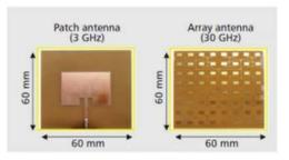
mmWave geometry allows for very small, high gain antennas
