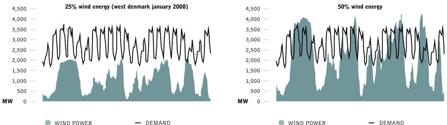
The left picture shows 25% wind energy in the Western Danish power system while the right picture shows 50% wind penetration (wind in grey/demand as orange line). It can be seen that with increasing penetration levels surplus wind power might be available at certain
