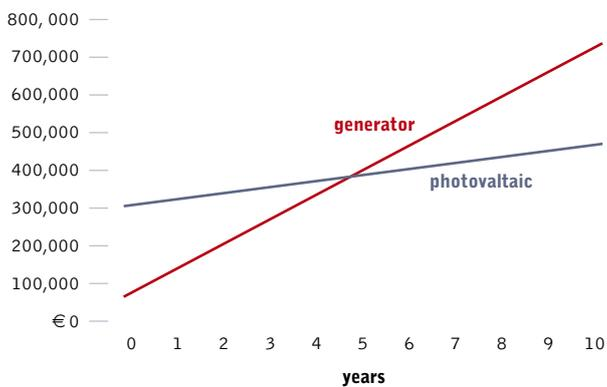
Case study Figure 2 shows the investment cost for a public grid extension versus an independent 30kWp photovoltaic power supply system. If we suppose a certain amount for a transformer station and 20,000 Euro per km of grid extension, the initial investment cost for a PV system is cheaper if it is situated further than 17 km away from the public grid.
