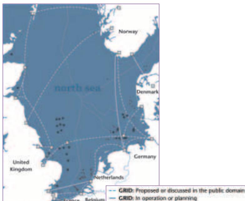
**KEY POINT:** An offshore grid may be more efficient than a series of one-off transmission link-ups, while interconnecting larger markets.
