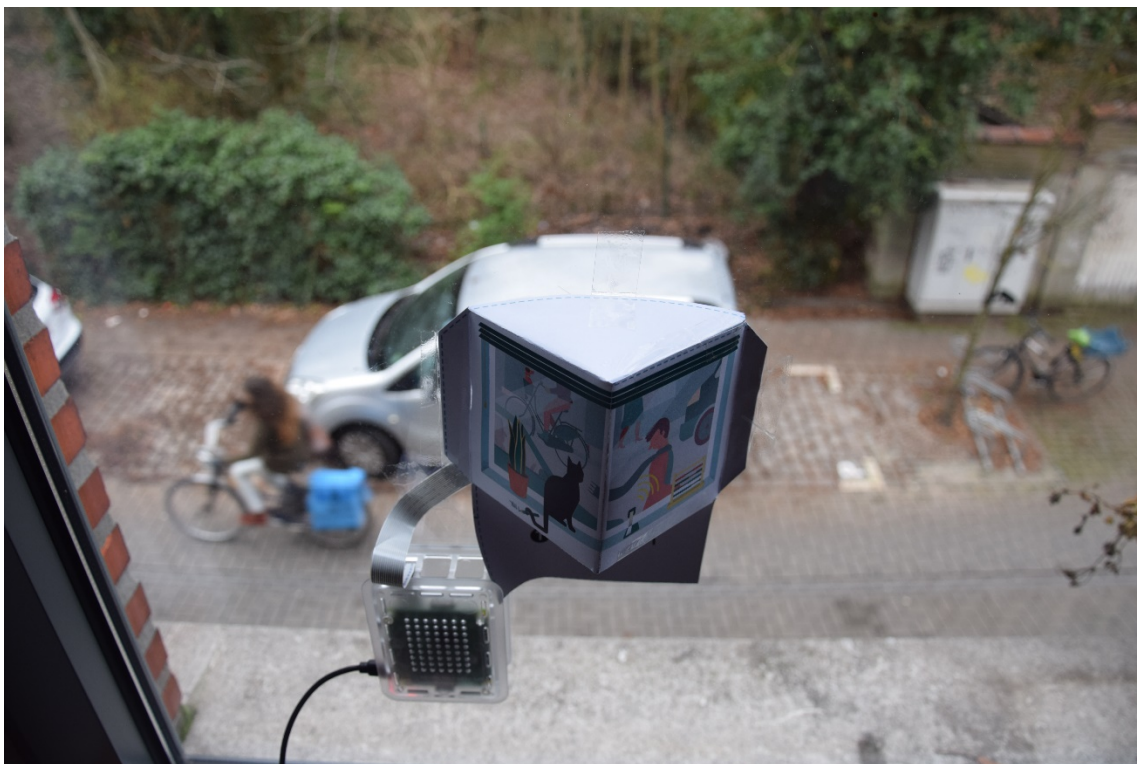
A tiny computer and camera attached to the window allow citizens to measure traffic in their street. Source: Telraam .
